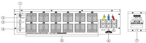
EMG/EXT (DC 12V~24V): Emergency/External start control. REM IN (DC 5V) for IR remote control input RS232 IN RS232 OUT 1~12 OUTLETS (Channel 1 ~12) Mains Connection Terminal Wiring Terminal Protective Shield
